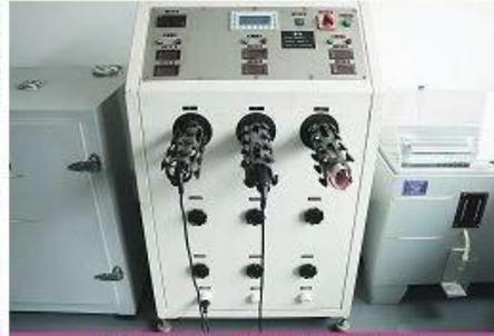
Power cord flexing test system
