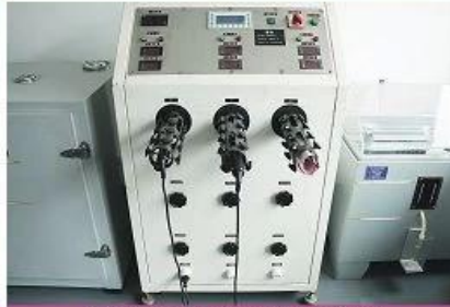
Power cord flexing test system
