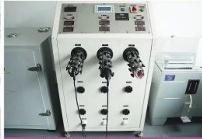
Power cord flexing test system
