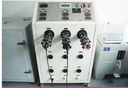
Power cord flexing test system
