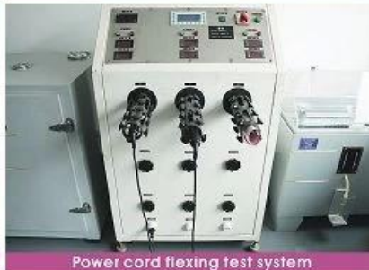
Power cord flexing test system
